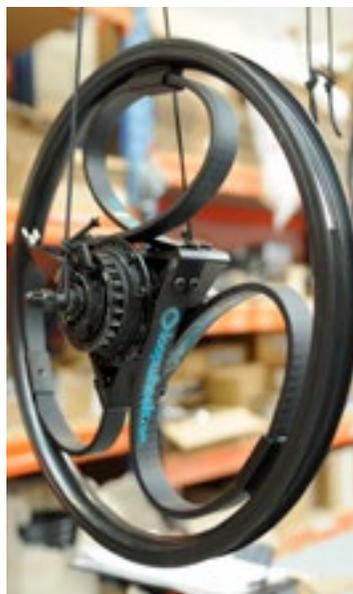
**ABOVE:** Rear wheel with Shimano Alfine 11-speed hub and Gates Carbon Drive sprocket.
